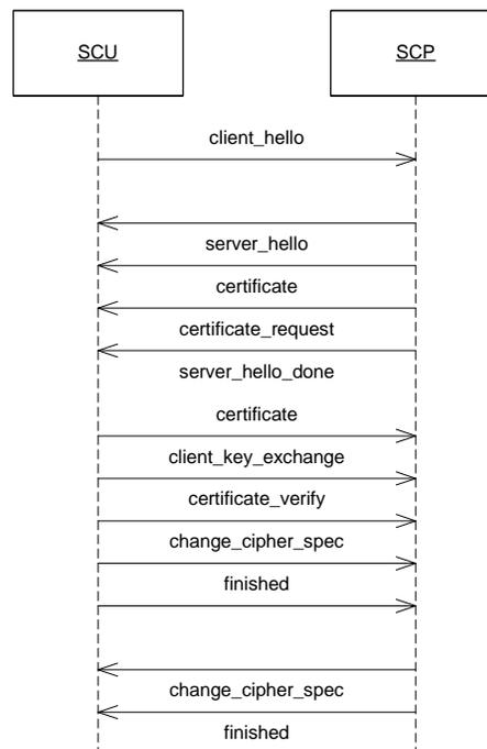
**Figure 20 Message flow of TLS handshake**
