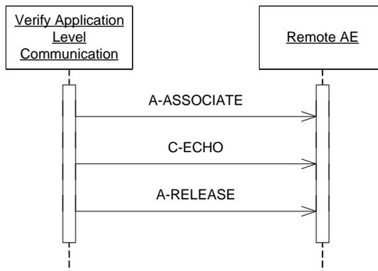
Figure 17 Sequencing of RWA Verify Application Level Communication
