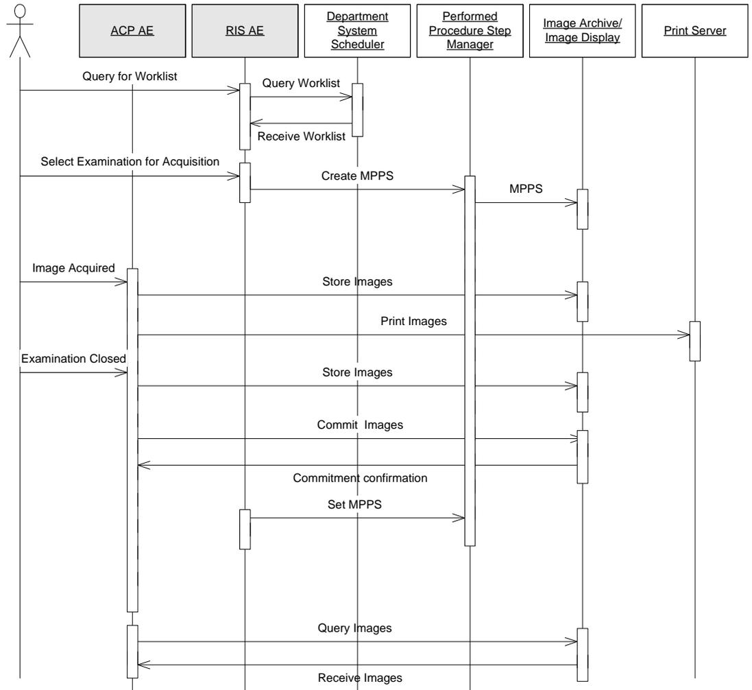
Figure 3 Allura Xper Sequencing constraints
