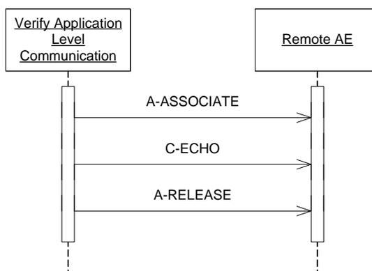
**Figure 7 Sequencing of RWA Verify Application Level Communication**
